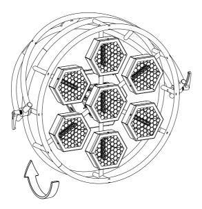
You can easily **change the orientation of tightened handles** to make your rig looks even better. Gently pull the tightened handle to disengage its teeth and rotate it into the desired orientation. By releasing the handle the return spring automatically engages the teeth.
