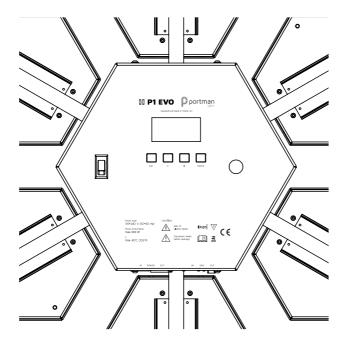
Navigation buttons are located under the OLED screen on the back panel. To enter the menu press the "Enter" button. To navigate the menu use the "+" and "-" buttons. To exit the menu from any level press "ESC". For confirming simply push the enter button. The buttons have descriptions under them. When you are in the main screen view, you can change the DMX address (if the DMX signal is present) or the brightness of the HaloLED sources (if there's no DMX) without entering the menu.
