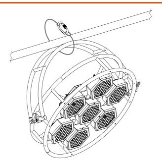
REMEMBER! Always secure hanged fixture with safety wire!
